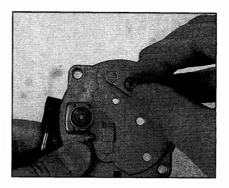
10. Install metering diaphragm and then gasket, aligning holes in diaphragm and gasket with pins.
