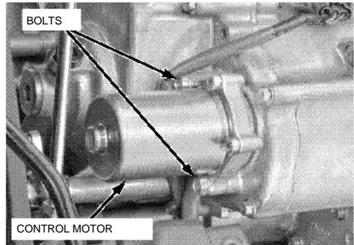
Coat a new O-ring with engine oil and install it into the control motor groove.
