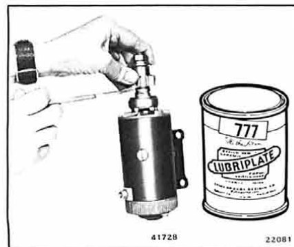
Figure 2-6. Starter Pinion Gear Shaft Helix
